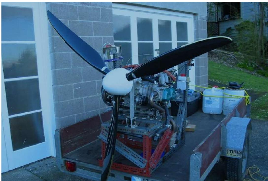
*“ .... planning on a modernised retake of the Ben Hur chariot race with a Rotax 912 ULS powered one. There have been a few teething problems as the high thrust line of the motor pulls the rear of the chariot down, in spite of 100lts of water in containers at the front, with disastrous consequences for the propeller tips ...”*
